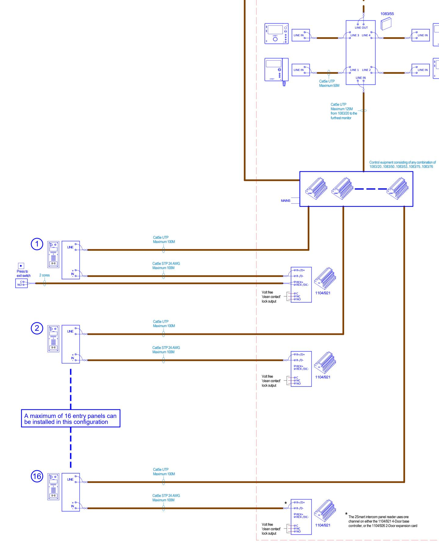
NOTES: 1. This schematic is for guidance only and should not be used for installation 2. Maximum distance from door entry panel to control equipment is 100m using Cat5e cable 3. Maximum distance from control equipment to the monitor is 125m using Cat5e cable 4. Maximum distance from 1083/55 to the monitor is 50m using Cat5e cable 5. Spare cores in Cat5e cable must not be used for other services -
