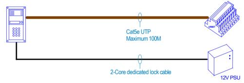
7. Add a second Cat5 cable if there is an Urmet/FDI access control reader fitted in the panel -
