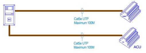
8. Cabling for double pole push to exit switch, double pole break glass unit and maglock -
