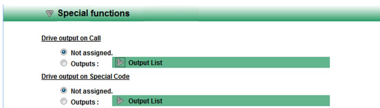
Figure 81: Advanced configuration – Special Decoder Functions that can be associated to the IP call module
