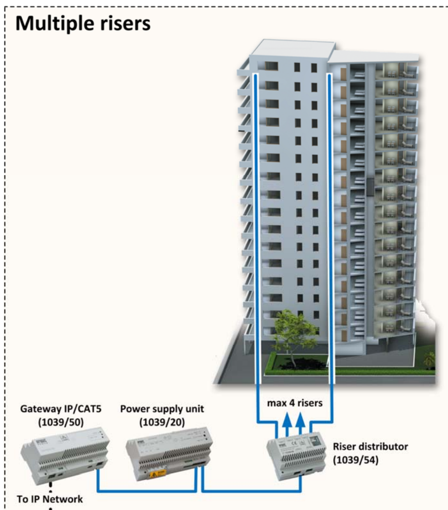
Figure 7: distribution on multiple CAT5 risers
