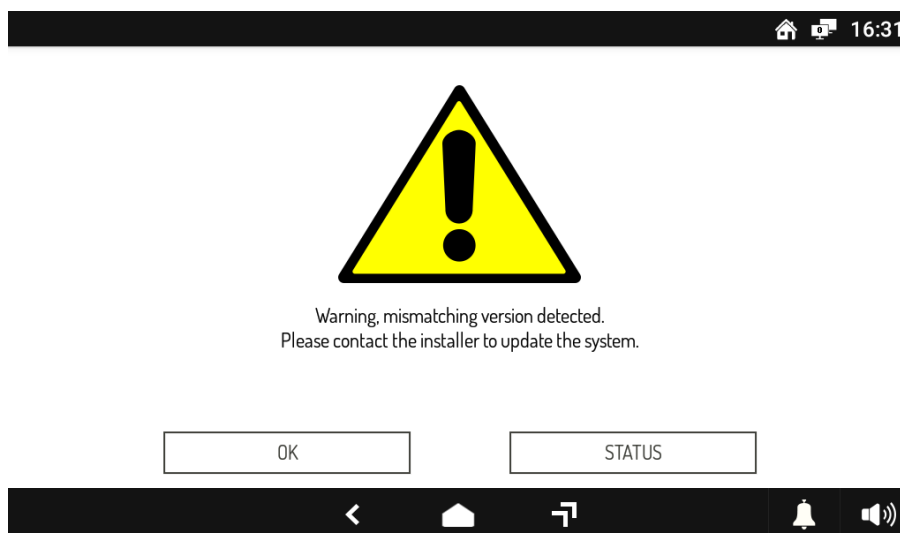
Figure 641: misalignment signalling on video door phone not present in the system configuration
