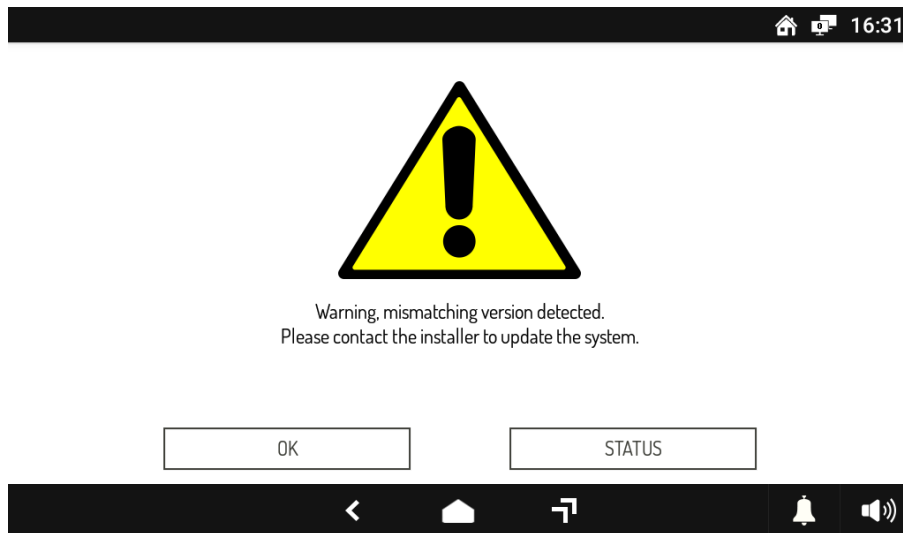
Figure 645: misalignment reporting on video intercom for Switchboard application not aligned with the UPTK version of the system
