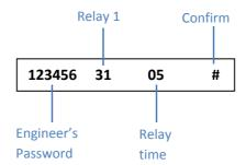
Wait 30 seconds for the keypad to exit from the programming mode.
