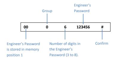
In summary move the **EXPL/PROG** jumper to the **PROG** position, press **00 0 6 123456** # then move the **EXPL/PROG** jumper to the **EXPL** position.
