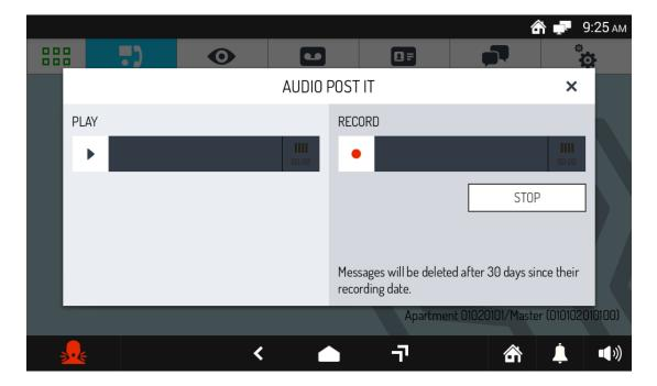
To record a new message open the pop-up window, tap the **RECORD** icon and start recording. The maximum permitted duration of the message is 10 seconds. The time to the end of recording is shown on a scroll bar.
