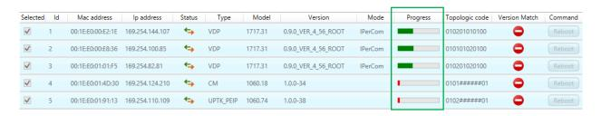
In the first phase Max video door phones upload the firmware upgrade file (green bars) while call modules and outdoor stations start the upgrade phase (red bars).
